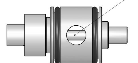
This is what you should see though the empty hole for the valve retention screw
